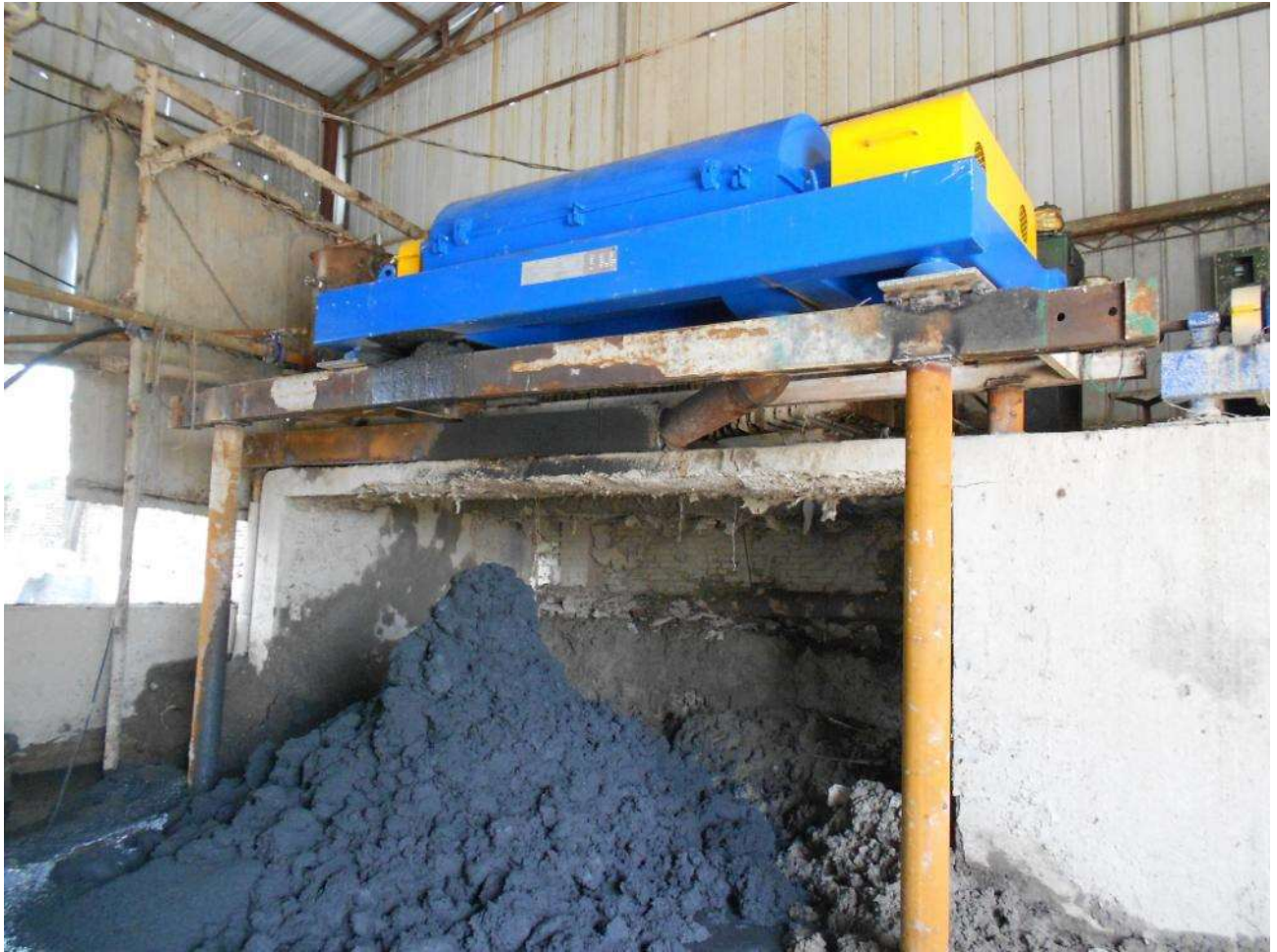
Figure 10: Centrifuge decanter using wastewater (Source: Sinoped)
