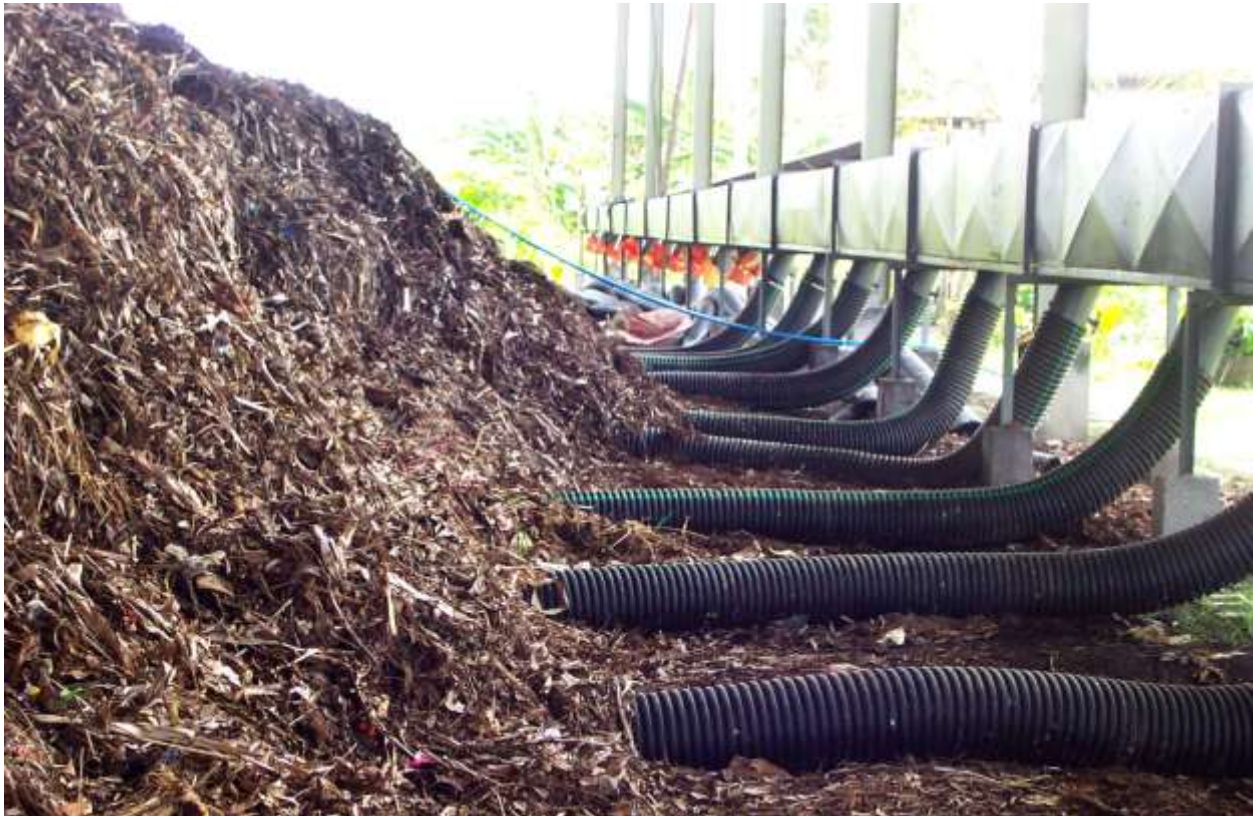
Figure 25: The biomass is aerated to ensure aerobic composting, resulting in the production of carbon dioxide and heat rather than methane (myclimate, 2017)
